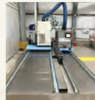
A flexible duct (in blue) to suck the fumes
