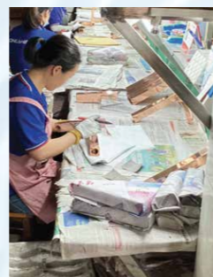
Electro-plating quality check. Any products found with a warping image will be ringed in red and rejected for a redo. They undergo at least 3 rounds of check
