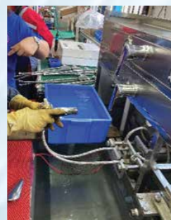
Water pressure applied to the faucet to check for leakage and strength of the correct pressure reading
